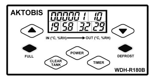
Once the construction dryer is properly connected to the socket, the backlight of the display panel lights up. After switching on the appliance (power), the LED display (detailed display) lights up automatically.
